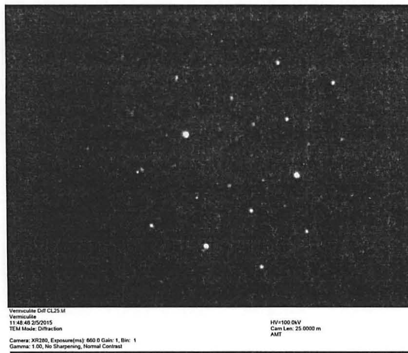
Figure 1. Electron diffraction pattern. (Used with the permission of Materials & Chemistry Laboratory, Inc.)
